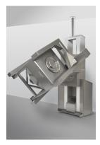
The square bin blender provides homogeneous blending of dry powder batches using patented blending elements mounted to the inside of the container lid. The blending procedure can be scaled from 400 to 2,600 liters. The blender can also accommodate loads up to 2,500 kg, depending on the model.
