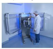
Operators will find the LM 40 modular, compact and easy to operate. It is designed as a mobile unit. The blender itself is integrated into a frame with locking castors. An interlocked Plexiglas cover protects the blending containers during rotation to ensure full safety during hazardous conditions. The blender has a drive unit with a bevel gear motor and potentiometer control to adjust the rotational speed.
